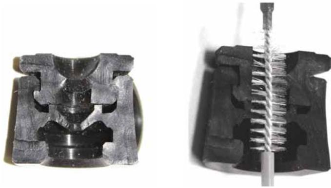
Figures 1 and 2 show a cross-sectional view of a typical biopsy port valve, demonstrating the nooks and crannies as well as the inability of a cleaning brush's bristles to contact all surfaces. *Photos courtesy of US Endoscopy*
